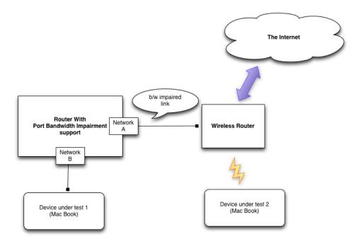
A special version of the Cisco router with pMod tool is used for impairing bandwidth between the networks to which devices under test are individually connected. The device under test (DUT) 1 is physically connected to "Network B", whereas, DUT-2 is wirelessly connected to Internet through Linksys wireless router. The router itself is connected to the wireless router via "Network A" a shown.
